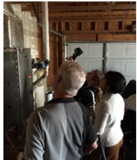
Photo: GOE staff and a Nevada Housing Division contractor use a thermal spectrometer to test heat loss at a State employee's home in Washoe County (Source: GOE).
