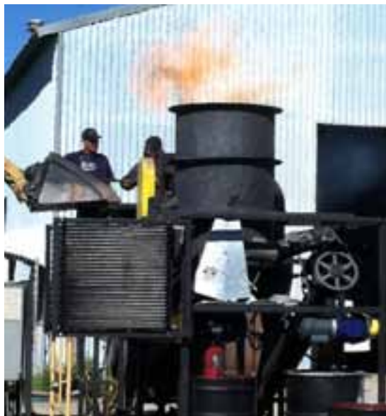
The kiln that converts pinyon juniper into bio-char, a charcoal used as a soil amendment. Image courtesy of Chris Lynch, University of Nevada Small Business Development Center.
